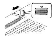
• Load a new paper stack only after the old one has run out.
